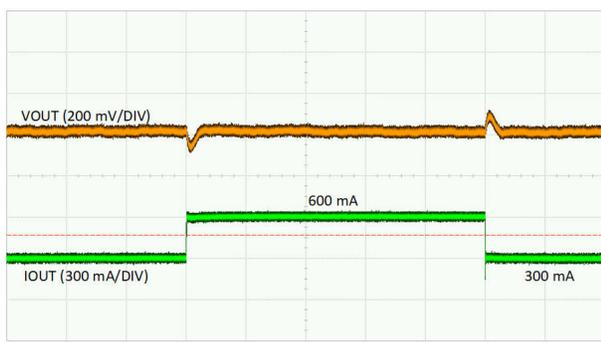
Figure 3-7. Load Transient 12V<sub>IN</sub>, 3.3V<sub>OUT</sub>, I<sub>OUT</sub> = 300mA to 600mA, Slew Rate = 1A/μs (FPWM)
