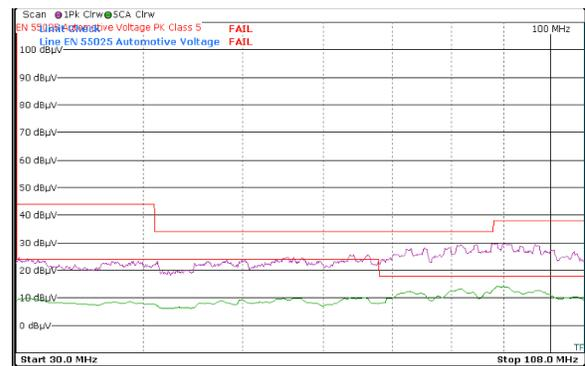
Figure 3-12. LMR43606MQ3EVM-2M High Frequency Conducted EMI Results
