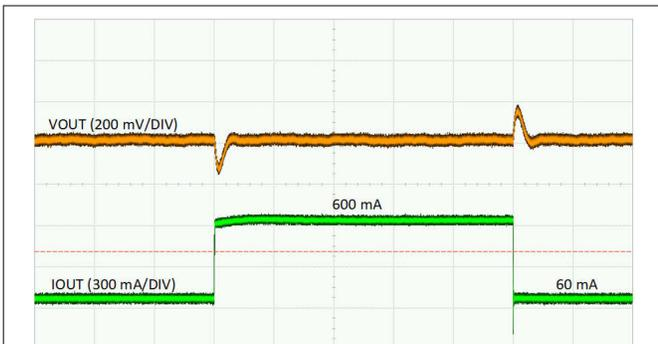
Figure 3-5. Load Transient 12V<sub>IN</sub>, 3.3V<sub>OUT</sub>, I<sub>OUT</sub> = 60mA to 600mA, Slew Rate = 1A/μs (FPWM)
