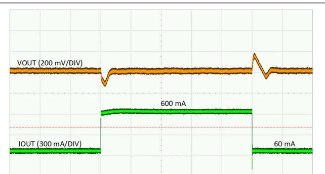
Figure 3-6. Load Transient 12V<sub>IN</sub>, 3.3V<sub>OUT</sub>, I<sub>OUT</sub> = 60mA to 600mA, Slew Rate = 1A/μs (AUTO)
