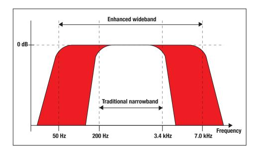
network. Even as digital technologies were introduced into telephony, the standard for voice remained the same voice quality of decades past, the quality produced by the analog phone network or PSTN – public switched telephone network. However, VoIP will soon join the HD parade as wideband codecs become widespread.
