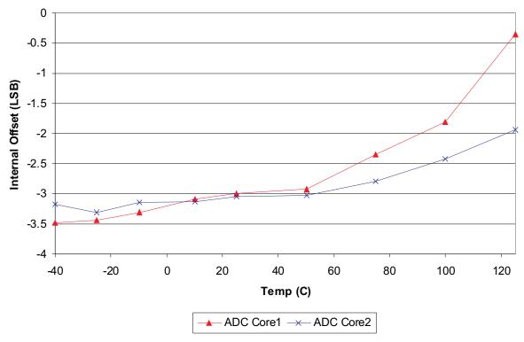
Figure 12. Internal Offset versus Temperate
