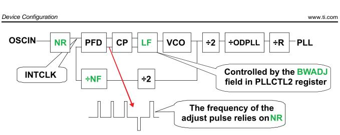
Figure 10. FMzPLL Block Diagram
