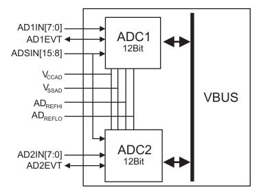
Figure 1. Channel Assignments of Two ADC Cores
