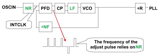
Figure 11. FPLL Block Diagram
