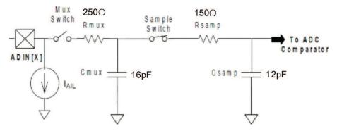
Figure 7. MibADC Input Equivalent Circuit
