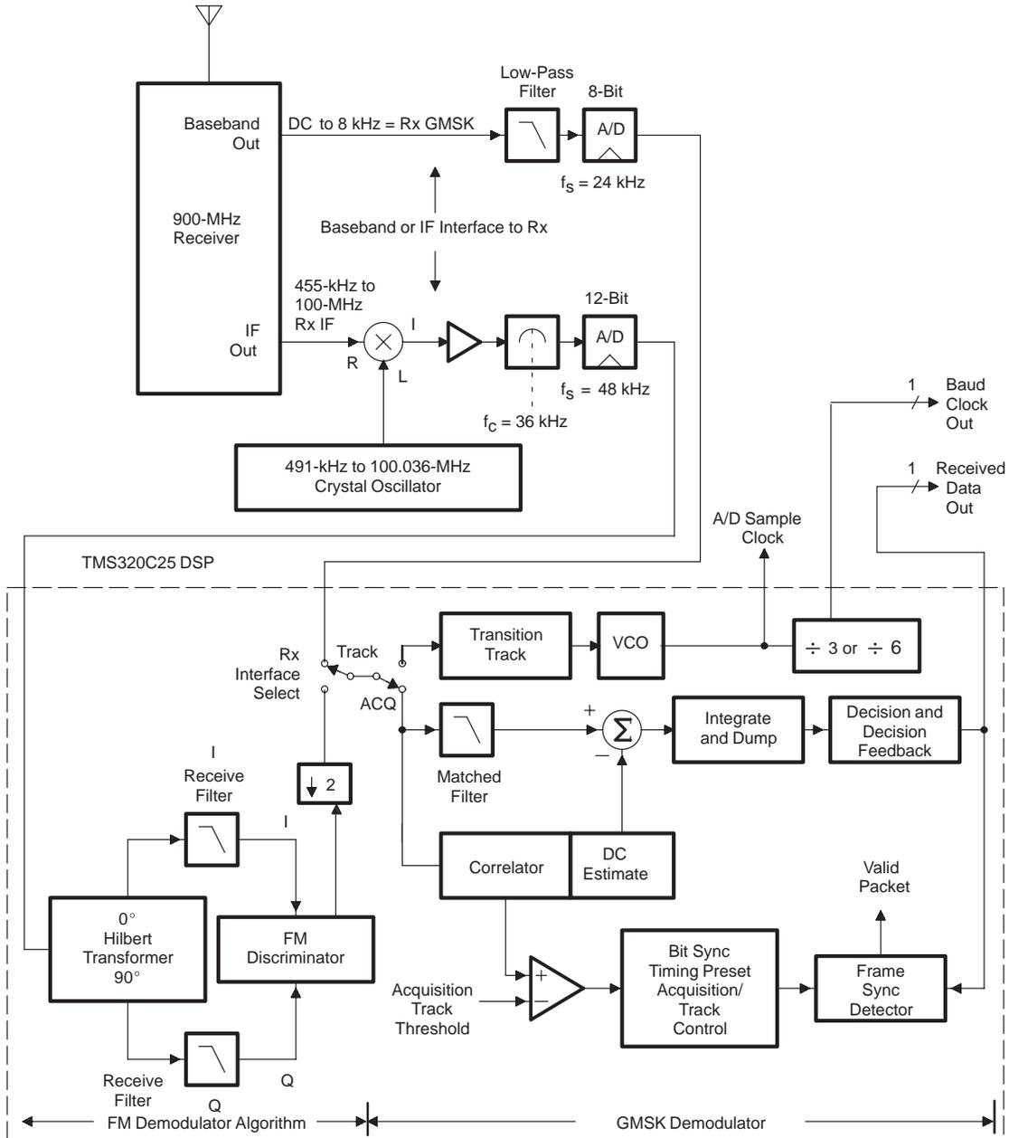
The demodulator algorithm employs noncoherent techniques to arrive at each data decision. Two entry points for digitized data from the receiver are shown in Figure 6.
