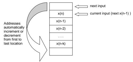
Since a great deal of software overhead is involved in checking the pointer values after every update, many DSPs provide circular buffering hardware that performs this function automatically. This hardware will wrap the pointer around once it goes past the end or start of the buffer.
