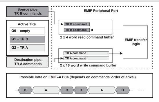
Figure 10. Parallel Read/Write Scenario
