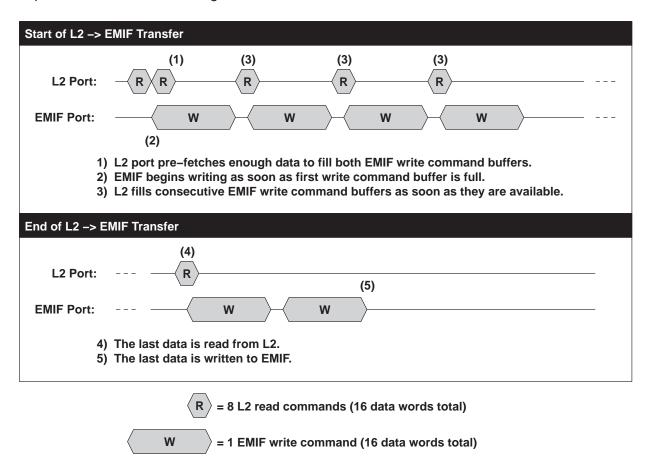
Figure 6. Port Activity is Determined by Command Buffers
