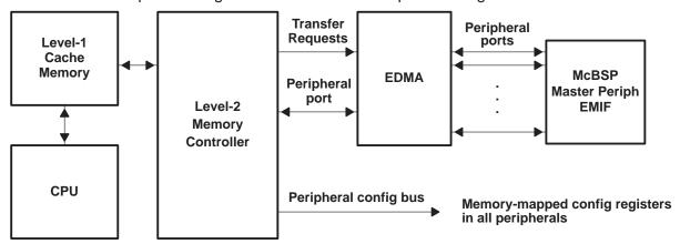
Figure 2. L2 Controller Functionality
