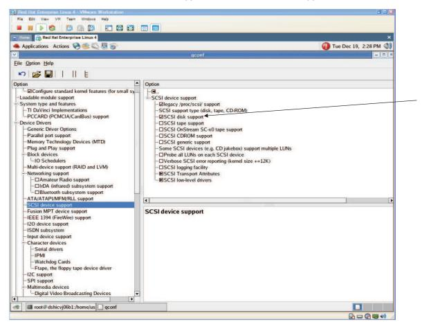
Figure 2. Xconfig Utility Showing How to Enable SCSI Disk Support
