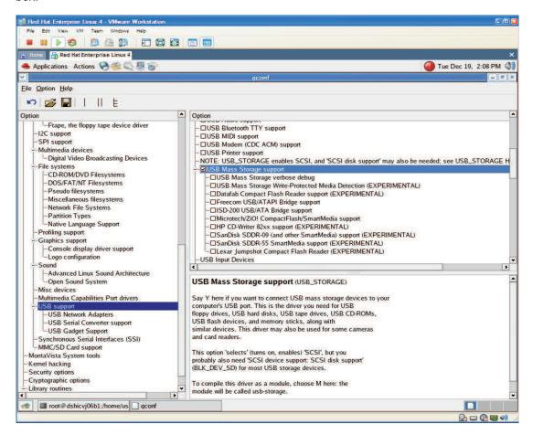
Figure 1. Xconfig Utility Showing How to Enable USB Host Mass Storage Support
