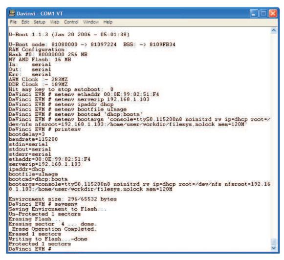
Figure 3. Tera Term Capture Showing How to Load Linux Kernel via TFTP
