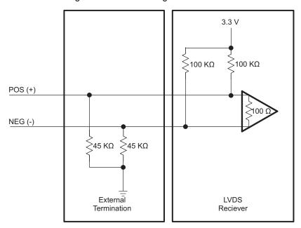
Figure 5. External Terminations: Receiver With 100  $\Omega$  and Pull-Ups
