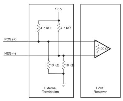
Figure 4. External Terminations: Receiver With 100  $\Omega$
