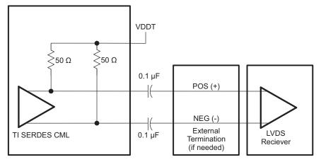
Figure 2. CML to LVDS Connection Basic Diagram
