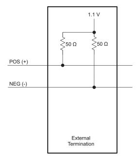
Figure 3. External Terminations: Receiver Has No Internal Terminations
