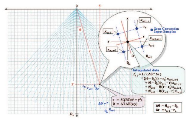
Figure 2. Scan Conversion Using Bilinear Interpolation for Sectored Image
