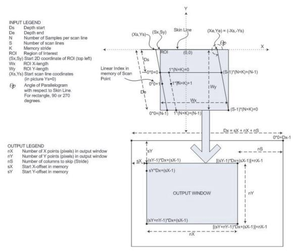
Figure 3. Input and Output Parameters of TI Scan Conversion API for Linear probe
