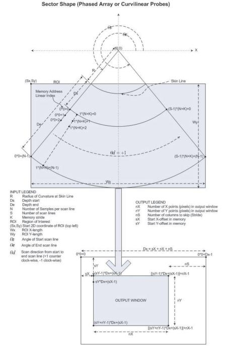
Figure 4. Input and Output Parameters of TI Scan Conversion API for Phased or Curvilinear Probe
