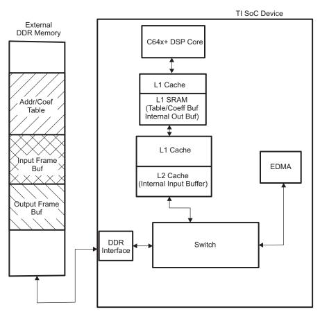
Figure 5. Block Diagram for TI Scan Conversion I/O Scheme
