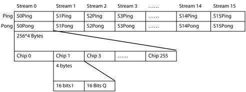
Figure 21 DL Type Data Buffer Structure Example in DSP Memory
