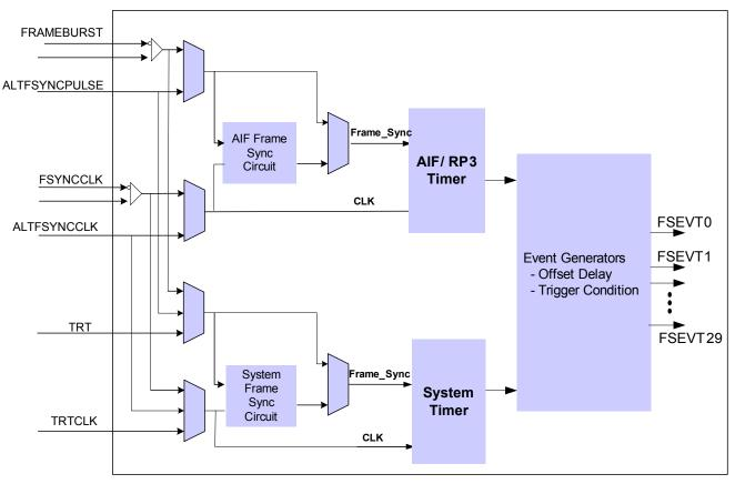
Figure 25 TCI648x FSync Block Diagram
