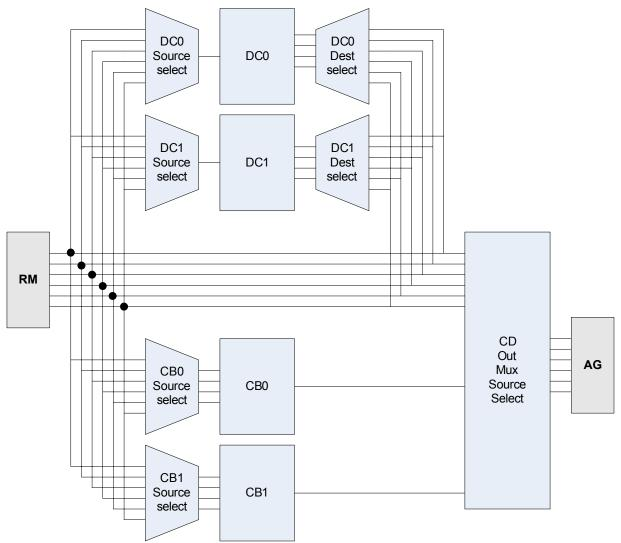
The main configuration for the CD are source/destination selections; most of these are straightforward. If decombining, each output mux source select used for decombining should select the same input link as the Decombiner. For example, if DC1 decombines input link 1 to link 2 and 3, the CD out mux source selection should be 1 instead of 2 or 3.
