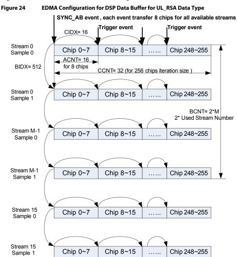
Figure 24 shows an EDMA transfer for a single link.
