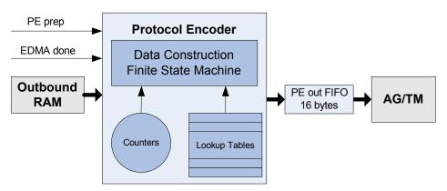
The PE prep tick from the FSync starts the PE, but real data processing happens only when:
