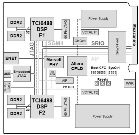
Figure 5 on page 7 shows the AIF connection between two DSPs on the TCI6488 EVM. The six AIF links are used to allow the following in the default configuration:
