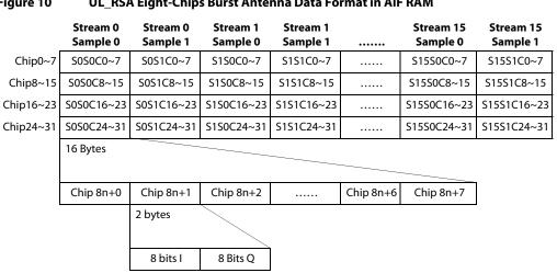
Figure 10 UL\_RSA Eight-Chips Burst Antenna Data Format in AIF RAM
