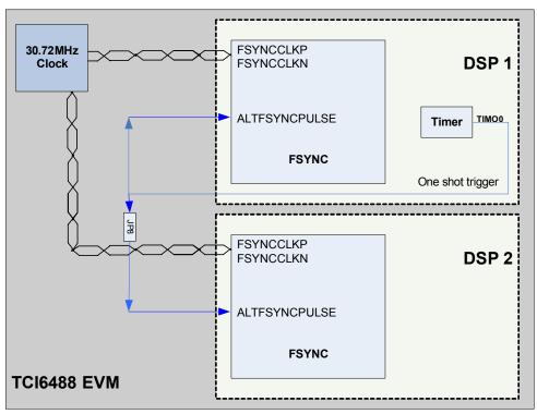
Figure 27 Synchronization of Two DSPs on the TCI6488 EVM
