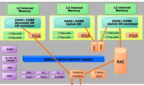
The integrated antenna interface (AIF) supports both OBSAI (Open Base Station Architecture Initiative) and CPRI (Common Public Radio Interface) standards, which interface with the IF/RF (Intermediate Frequency/ Radio Frequency) module for antenna data transfer. The AIF transfers baseband IQ data with a high-speed SERDES interface.
