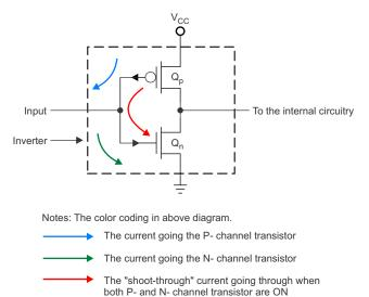
Figure 5. CMOS I/O
