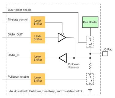
Figure 8. Typical I/O Cell
