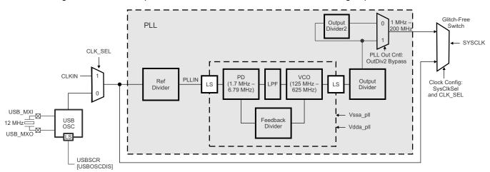
Figure 2. System Clock Generation - C5517
