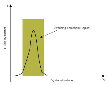
Figure 6. Switching Threshold Region
