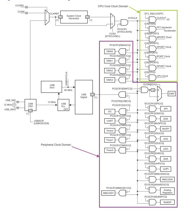
Figure 4. C5517 Clock Diagram
