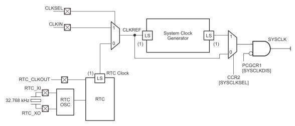
Figure 1. System Clock Generation - C55x5
