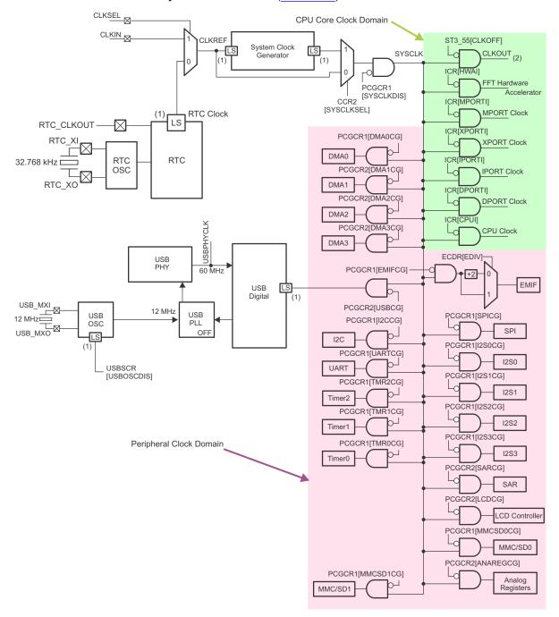
Figure 3. C55x5 Clock Diagram
