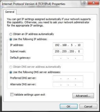
Figure 5. Static IP Configuration on Host PC
