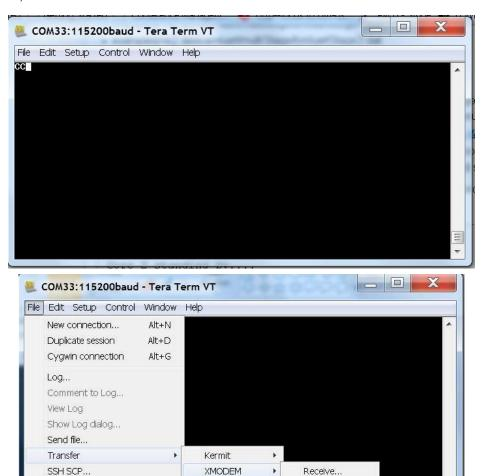
Figure 4. Teraterm Serial Terminal Usage for XMODEM Transfer of UART Boot Image
