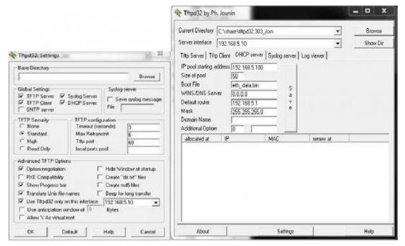
Figure 6. TFTP Transfer Configuration for Ethernet Boot
