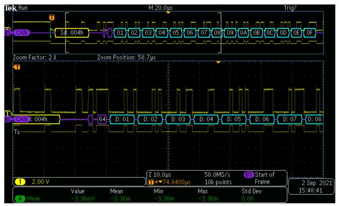
Figure 3-4. Output From MCANTX Pin for mcan\_ex3\_transmit.c
