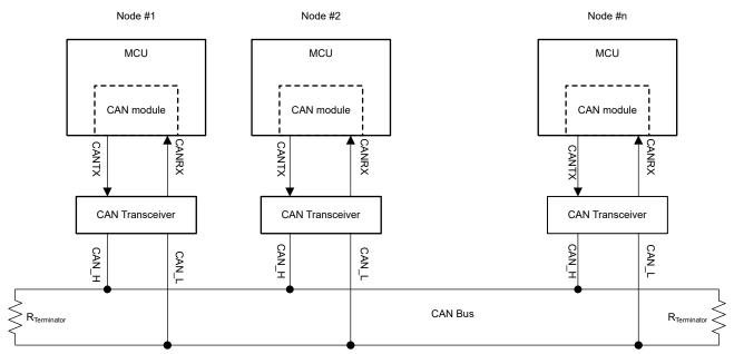
Figure 1-1. Typical CAN bus
