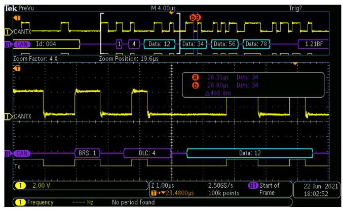
Figure 3-1. Output From MCANTX Pin for mcan\_ex1\_loopback.c
