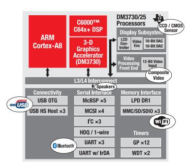
ARM processor through a set of easy-to-use application programming interfaces (APIs). The DSP library contains more than 80 algorithms, including multi-media decoders and encoders, math functions, digital filtering including Fast Fourier Transform (FFT), and image processing including image filtering and analysis.
