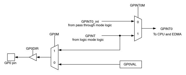
When GP0 is configured as an output (GP0DIR = 1), the GP0M bit controls whether the GP0 signal operates in GPIO mode or in logic mode. In GPIO mode (GP0M = 0), the value of the GP0VAL bit is driven out on GP0. In logic mode (GP0M = 1), GPINT is driven out on GP0. When GP0 is configured as an input, GP0M has no effect.
