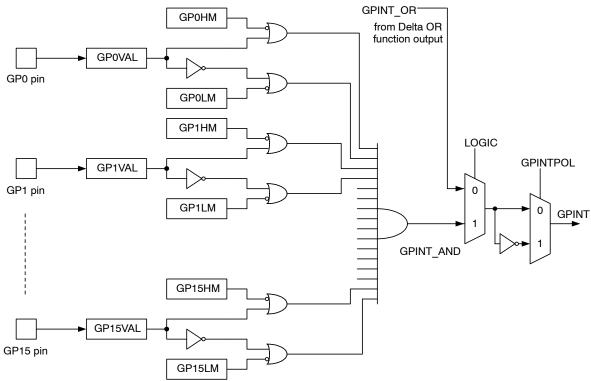
**Note:** The functional block diagram shows the mask logic as an OR with an inverter on the mask bit. This forces the OR to evaluate true when the mask bit is disabled. This is strictly a functional block diagram. The actual implementation prevents the GPINT from being asserted in the case that all the mask bits are disabled.
