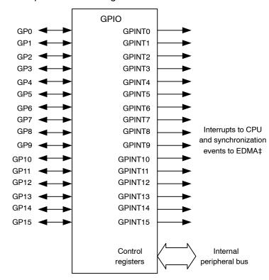
Figure 2. GPIO Peripheral Block Diagram
