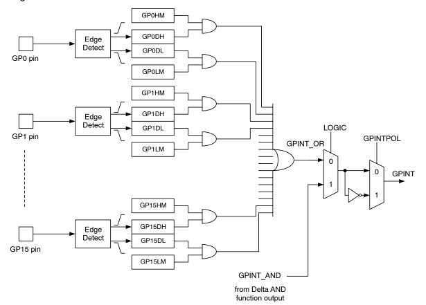
Figure 7. GPINT Generation in Delta OR Mode
