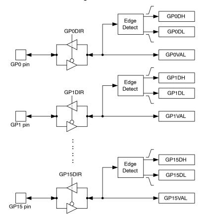
Figure 3. GPIO Functional Block Diagram
