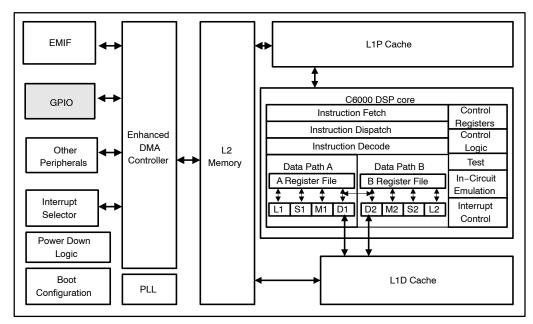
Some GPIO pins are MUXed with other device pins. On a given device, all bits may not be implemented for each GPIO register. Refer to the device-specific datasheet for details on specific MUXing and for the availability of the register bits. GPINT[0–15] are all synchronization events to the EDMA. However, only GPINT0 and GPINT[4–7] are available as interrupt sources to the CPU.
