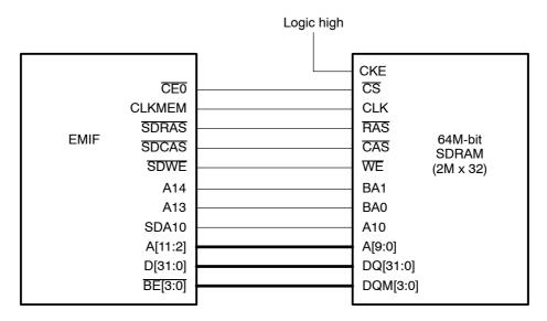
Table 4–4. EMIF Configuration for a 64M-bit SDRAM Chip With a 2M x 32 Array Organization
