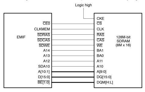
Figure 4–5. Interfacing to a 128M-bit SDRAM Chip With an 8M x 16 Array Organization
