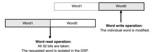
For a read operation, the EMIF uses the full data bus, D[31:0], and drives all four byte enable signals low (active). For a write operation, the EMIF uses bit 1 of the internal address to determine which half of the data bus is used and which byte enable signals are active (see Table A–3 and Figure A–8).
