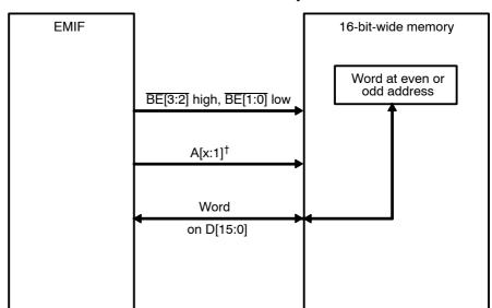
Figure A-9. 16-Bit Data Access of 16-Bit-Wide External Memory
