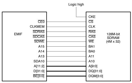
Figure 4-6. Interfacing to a 128M-bit SDRAM Chip With a 4M x 32 Array Organization
