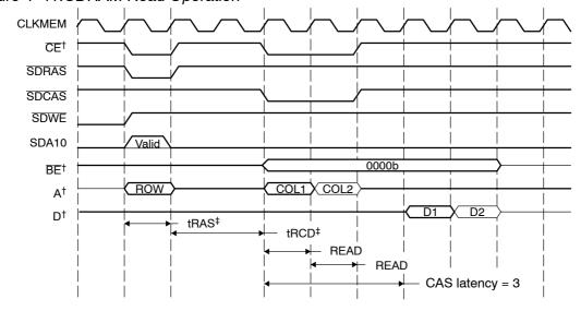
Figure 4-11.SDRAM Read Operation
