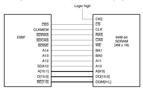
Figure 4–1. Interfacing to a 64M-bit SDRAM Chip With a 4M x 16 Array Organization
