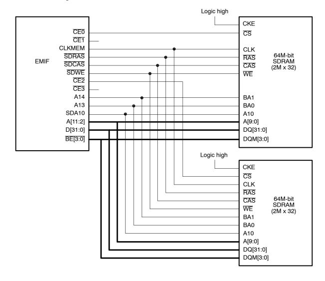
Table 4–5. EMIF Configuration for Two 64M-bit SDRAM Chips, Each With a 2M x 32 Array Organization
