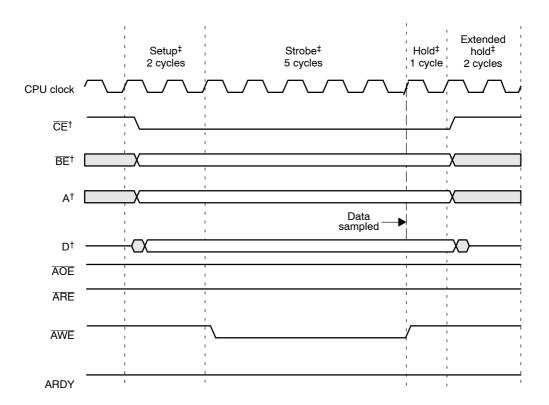
Figure 2-3. Asynchronous Write Operation
