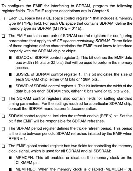
write to MEMFREQ to select the relative frequency of the memory clock signal. After programming MEMFREQ and the DSP clock
