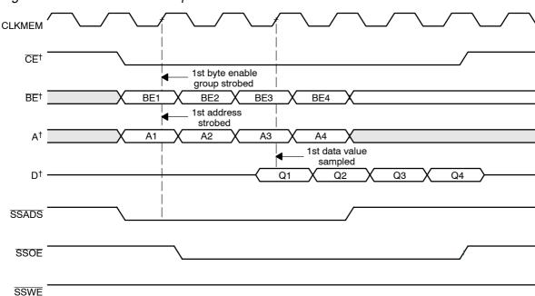
Figure 3-4. SBSRAM Read Operation
