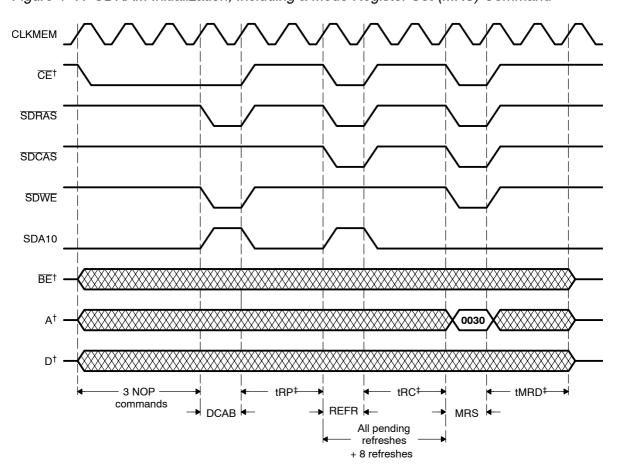
Figure 4-7. SDRAM Initialization, Including a Mode Register Set (MRS) Command
