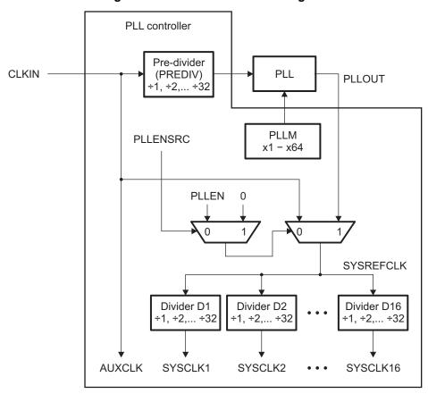
Figure 1. PLL Controller Block Diagram
