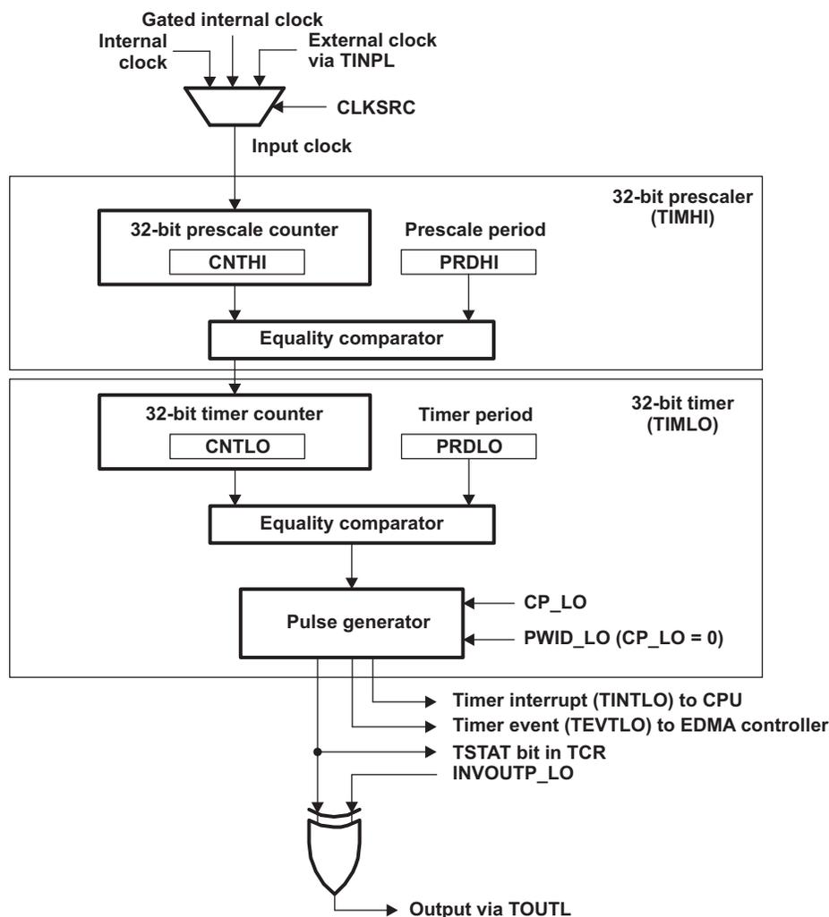
**Figure 5. Dual 32-Bit Timers Chained Mode Example**
