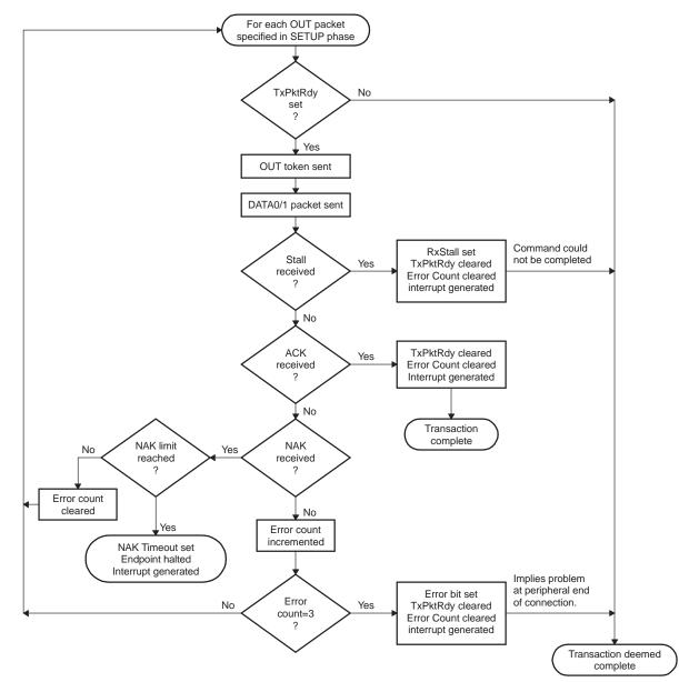
Figure 11. OUT Data Phase Flow Chart
