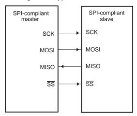
Figure 33. Typical SPI Interface
