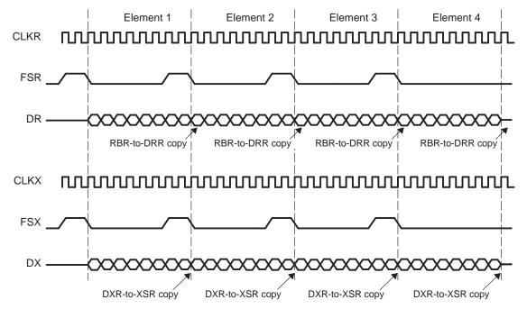
Figure 18. Maximum Frame Frequency Operation With 8-Bit Data
