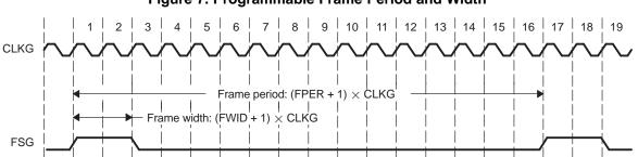
Figure 7. Programmable Frame Period and Width
