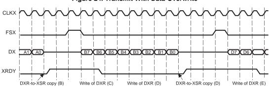
Figure 24. Transmit With Data Overwrite
