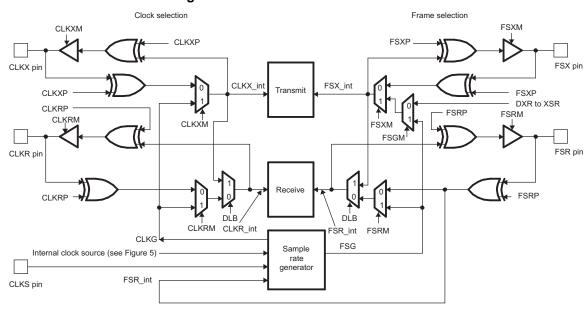
Figure 2. Clock and Frame Generation
