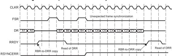
Figure 23. Unexpected Receive Frame Synchronization Pulse
