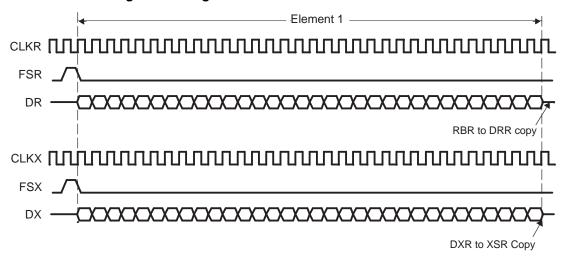
Figure 10. Single-Phase Frame of One 32-Bit Element
