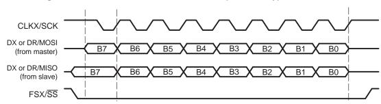
Figure 37. SPI Transfer With CLKSTP = 3h (clock delay) and CLKXP = 1
