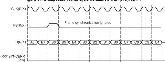
Figure 17. Unexpected Frame Synchronization With (R/X)FIG = 1
