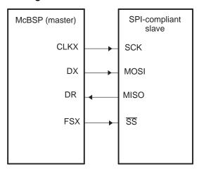
Figure 38. ASP as the SPI Master
