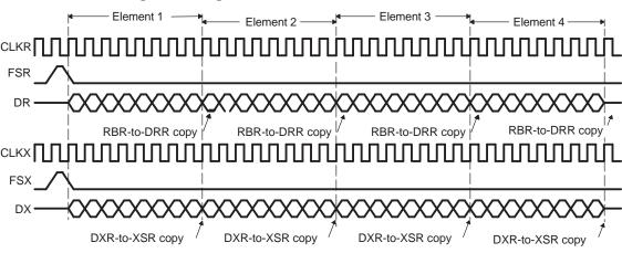
Figure 9. Single-Phase Frame of Four 8-Bit Elements
