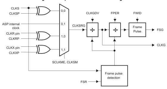
Figure 5. Sample Rate Generator Block Diagram
