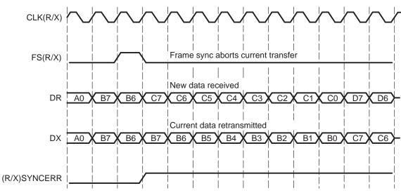
Figure 16. Unexpected Frame Synchronization With (R/X)FIG = 0
