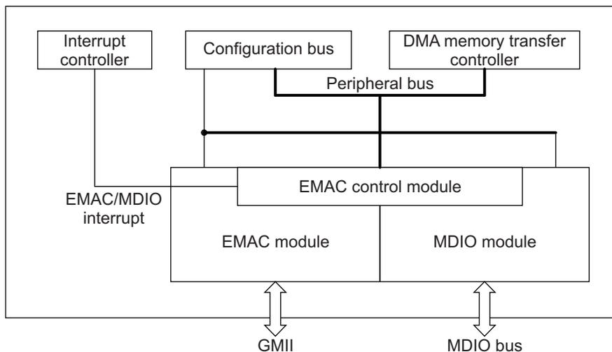
Figure 1 shows the main interface between the EMAC control module and the CPU. The following connections are made to the device core:
