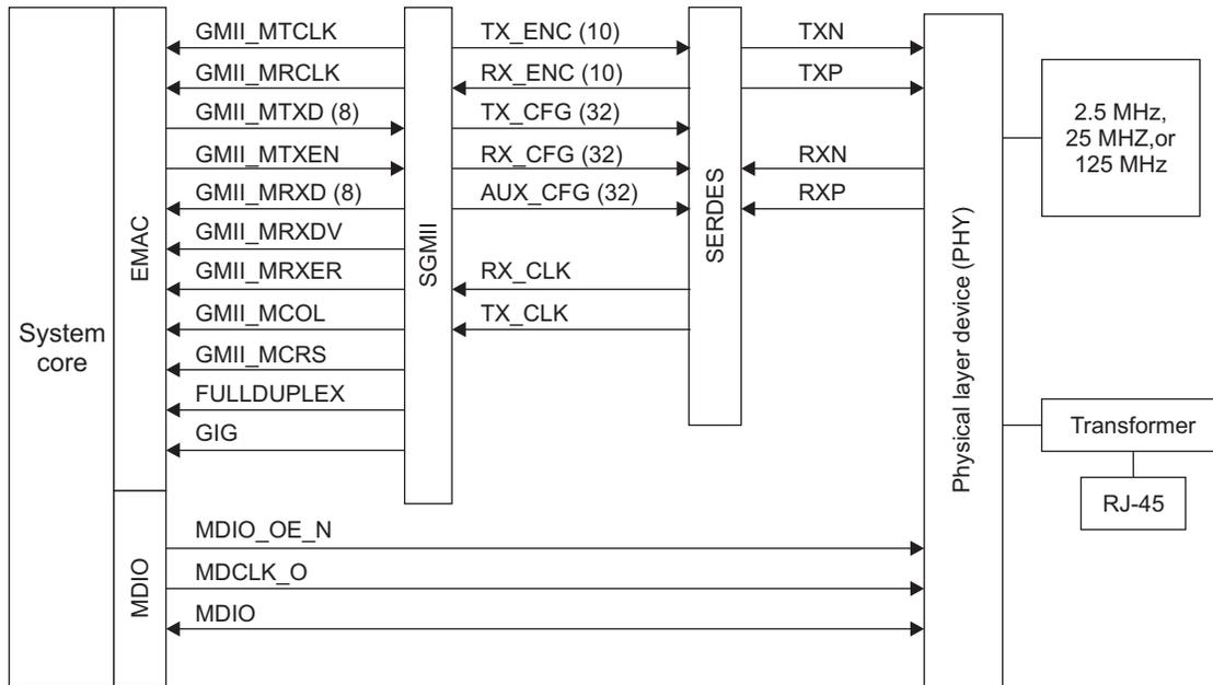
The SGMII interface supports 10/100/1000 Mbps modes. Only full-duplex mode is available in 1000 Mbps mode. In 10/100 Mbps modes, the GMII interface acts like an MII interface, and only the lower 4 bits of data are transferred for each of the data buses.
