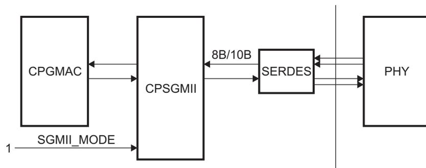
The following setup shows the CPSGMII setup for this mode of operation:
