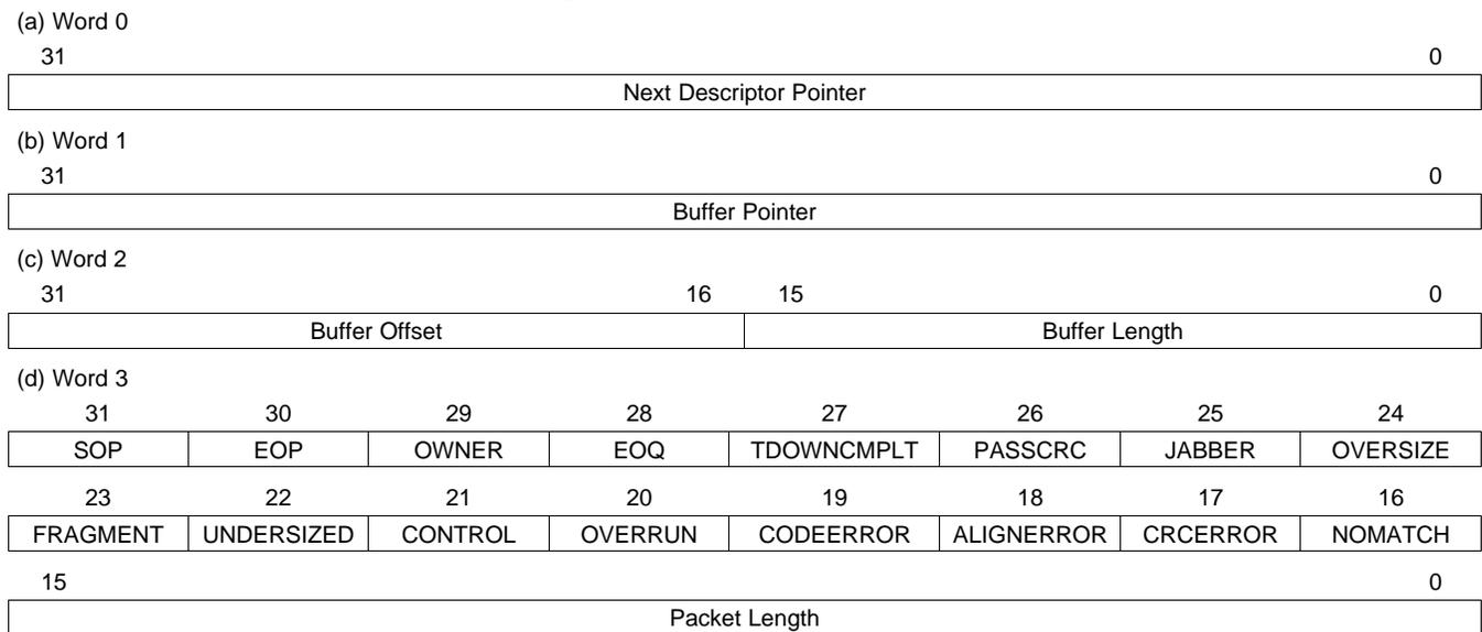
**Example 2. Receive Descriptor in C Structure Format**
