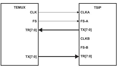
Figure 20. TSIP Connected to TEMUX
