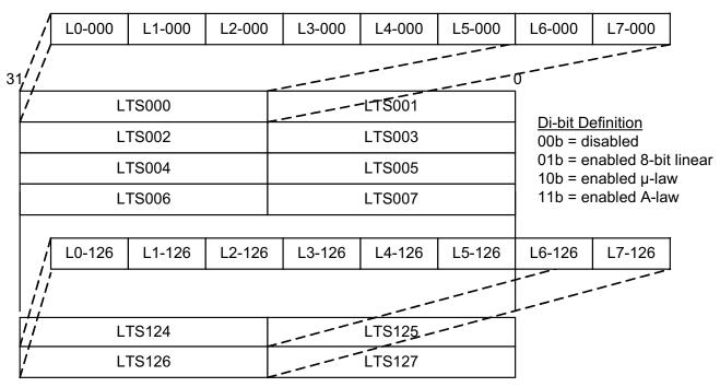
Figure 4. 8 Mbps Channel Definition (8 Links with 8 Active Links)
