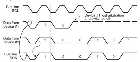
Figure 12. Arbitration Procedure Between Two Master-Transmitters
