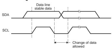
Figure 5. Bit Transfer on the I2C-Bus
