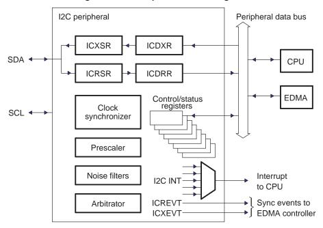
Figure 1. I2C Peripheral Block Diagram
