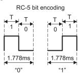
Figure 10. RC-5 Bit Encoding
