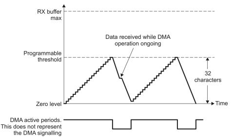
Figure 21. Receive FIFO DMA Request Generation (32 chars)
