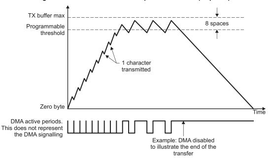
Figure 23. Transmit FIFO DMA Request Generation (8 spaces)
