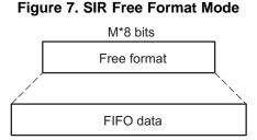
In this mode, the entire FIFO data packet is constructed (encoded and decoded) by the LH software.
