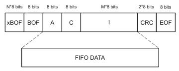
Figure 6. IrDA SIR Frame Format
