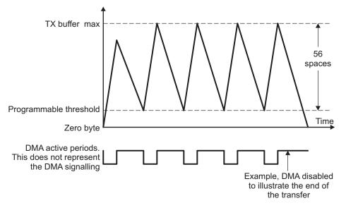
The DMA request is again asserted if the FIFO is able to receive the number of bytes defined by the TLR register (refer to Table 42).
