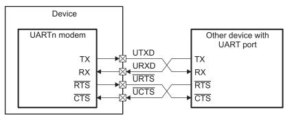
Figure 2. UART Modem Application Example
