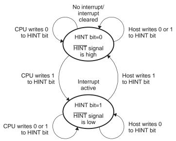
Figure 10. CPU-to-Host Interrupt State Diagram
