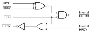
Strobe connections between the host and the HPI depend in part on the number and types of strobe pins available on the host. Table 2 describes some options for connecting to the HDS pins.
