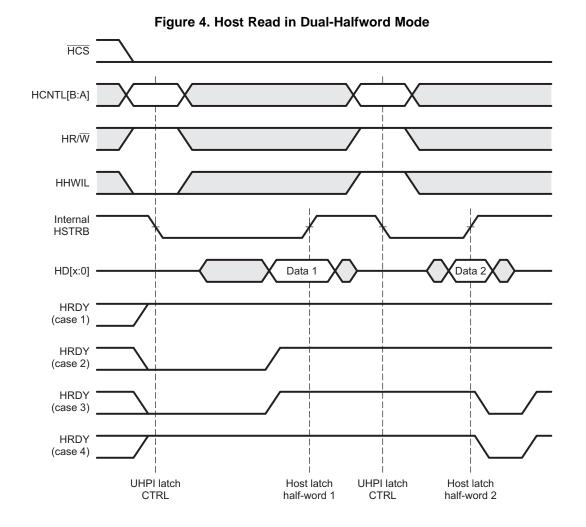
HRDY behavior will vary depending on the cycle type and previous conditions. There are four possible cases of HRDY behavior. In every case, HRDY may be initially de-asserted due to prefetch or memory write activity caused by the previous cycle. HRDY behavior is illustrated in Figure 4 and described below:
