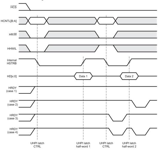
Figure 5. Host Write in Dual-Halfword Mode
