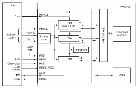
Figure 1. HPI Block Diagram
