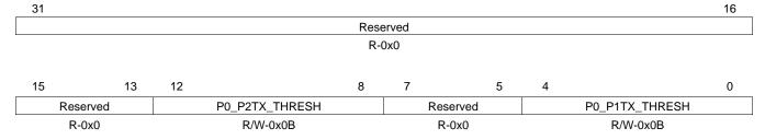
Table 16. 3pGSw Port 0 Flow Control Threshold Register (P0\_FLOW\_THRESH) Field Descriptions
