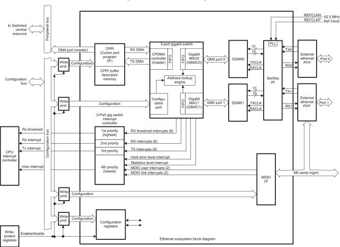
Figure 1. 3PSW Block Diagram
