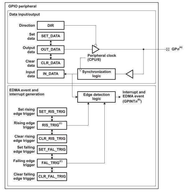
Figure 2. GPIO Peripheral Block Diagram
