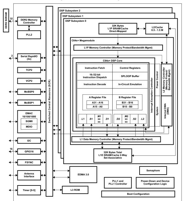
Figure 1. C6474 DSP Block Diagram
