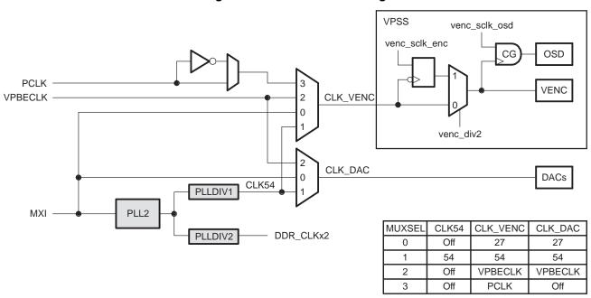
The 4 DACs are hooked up to the VENC module that is inside the Video Processing Back End (VPBE). The data flow between the VPBE and DACs is synchronous. The various possible clocking modes are shown in Figure 5-2 and described in Table 5-5.
