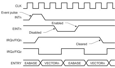
Figure 9-3. Immediate Interrupt Disable/Enable
