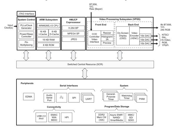
Figure 1-1. TMS320DM357 DMSoC Block Diagram
