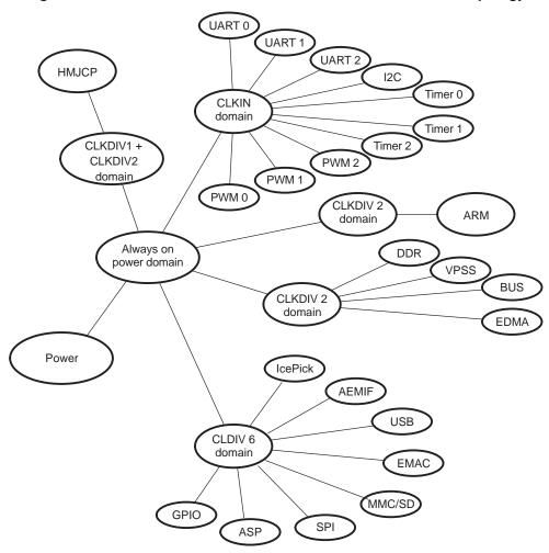
Figure 7-2. TMS320DM357 DMSoC Power Domain and Module Topology
