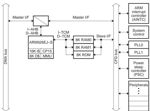
Figure 2-1. TMS320DM357 DMSoC ARM Subsystem Block Diagram
