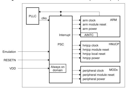
Figure 7-1. TMS320DM357 DMSoC Power and Sleep Controller (PSC)
