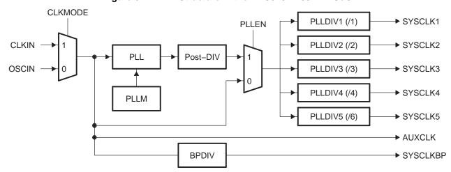
Figure 6-1. PLL1 Structure in the TMS320DM357 DMSoC
