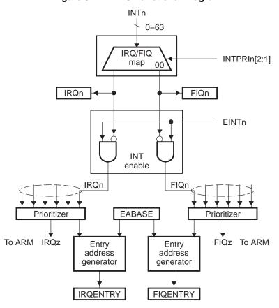
Figure 9-1. AINTC Functional Diagram
