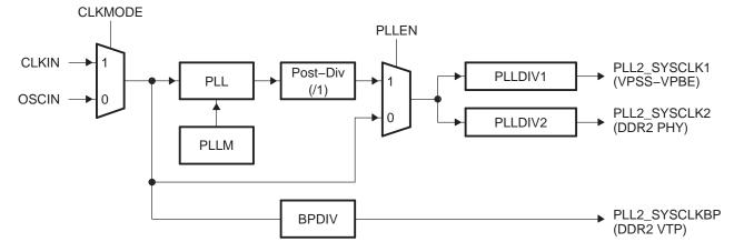
Figure 6-2. PLL2 Structure in TMS320DM357 DMSoC
