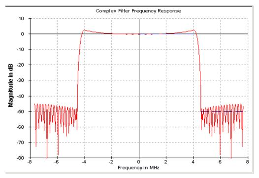
Figure 2-11. Example 79 Tap – Low Pass Filter Used for LTE10, with CIC Droop Compensation
