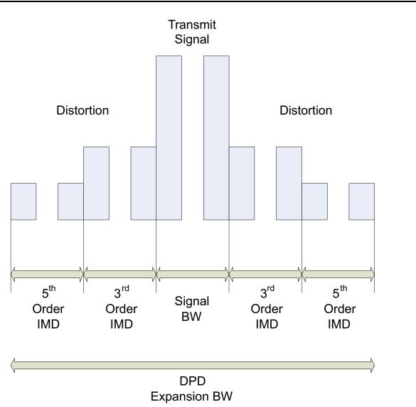
Figure 2-25. Transmit Bandwidth and DPD Expansion Bandwidth Example.
