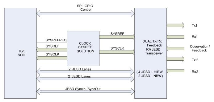
Figure 1-14. TCI663xK2L DFE to Two Antenna JESD Transceiver Block Diagram
