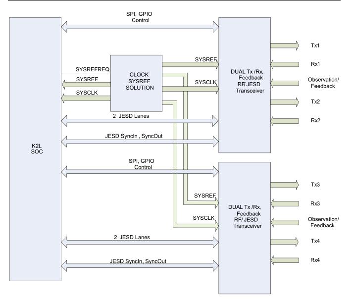
Figure 1-15. TCI663xK2L DFE to Four Antenna JESD Transceiver Block Diagram
