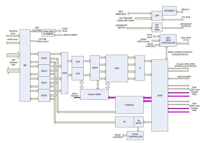
Figure 2-35. DFE Block Diagram for Feedback
