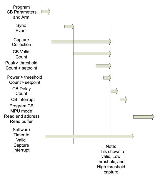
Figure 2-39. Capture Buffer Qualified Collection with Delay
