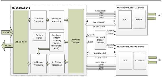
Figure 1-7. DFE with Discrete DAC and ADC
