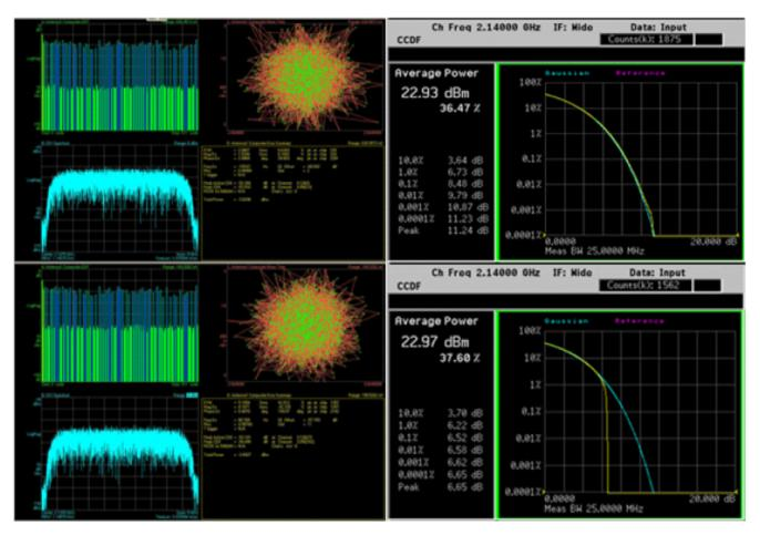
Figure 2-15. Effect of CFR on TX Antenna Carrier Signal (Upper-Before CFR/ Below after CFR)
