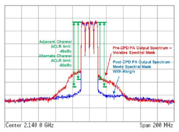
Figure 2-26. DPD Correction Showing Spectral Emission Mask Improvement
