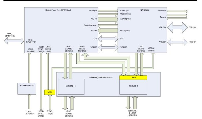
Figure 1-13. Boot Mode Shared Data Multiplexers IQNet and DFE
