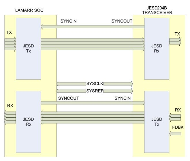
Figure 2-30. JESD Clock, Synchronization, and SerDes Data Diagram
