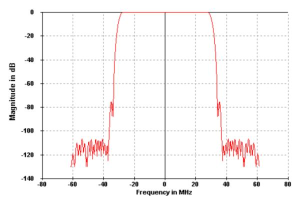
Figure 2-33. Example F2 Filter Decimate-by-Two Response, Sampled at 122.88 Mhz
