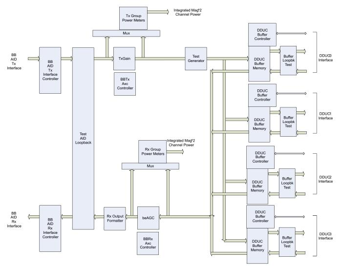
Figure 2-4. BB Block Diagram
