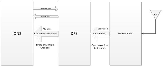
Figure 1-5. DFE RX Signal Processing
