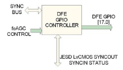
Figure 2-40. DFE GPIO Block Diagram
