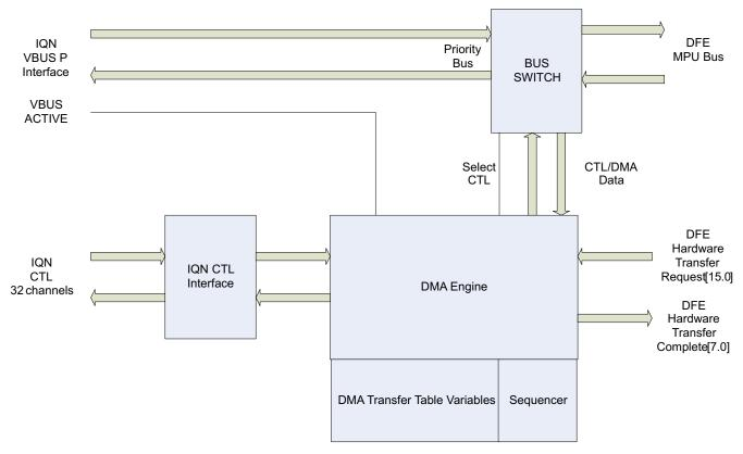
Figure 2-41. VBUSP2MPU CPP Sub-Block Diagram
