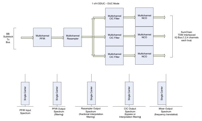
Figure 2-8. DDUC as a Digital Up Converter (1 Carrier Shown) Block Diagram
