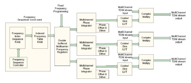
Figure 2-12. Multichannel Complex Mixer (3 Sections Shown)
