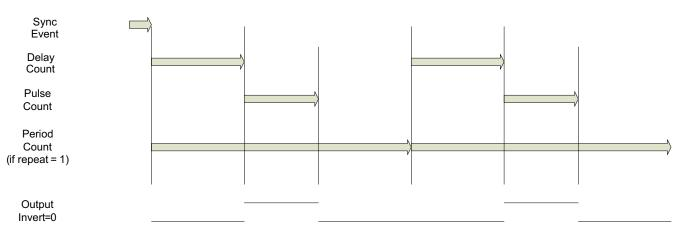
Figure 2-42. Sync Counter Operation
