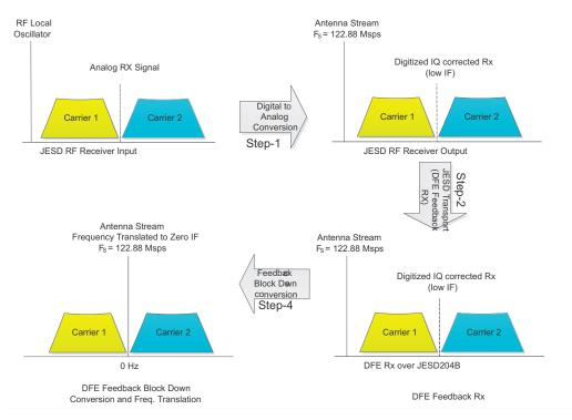
Figure 1-12. DFE Feedback RX Processing
