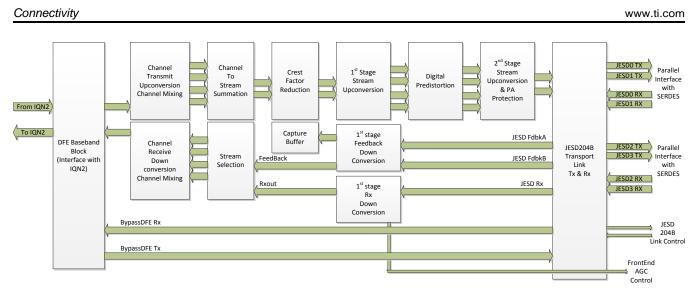
Figure 1-2. DFE Block Diagram
