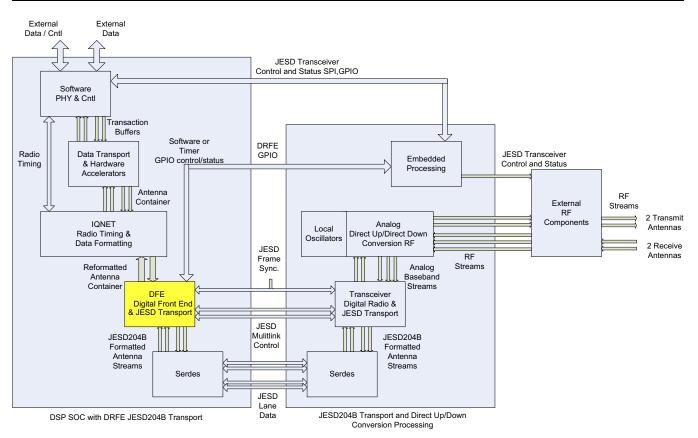
Figure 1-3. DSP SoC to JESD Transceiver SoC Flow and Control Diagram
