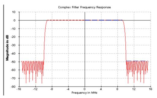
Figure 2-10. Example 79 Tap – Low Pass Filter Used for LTE20 Application
