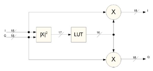
Figure 2-20. Circular Limiter Diagram
