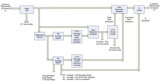
Figure 2-28. TX Sub-Block PA Protection (1 of 2) Diagram
