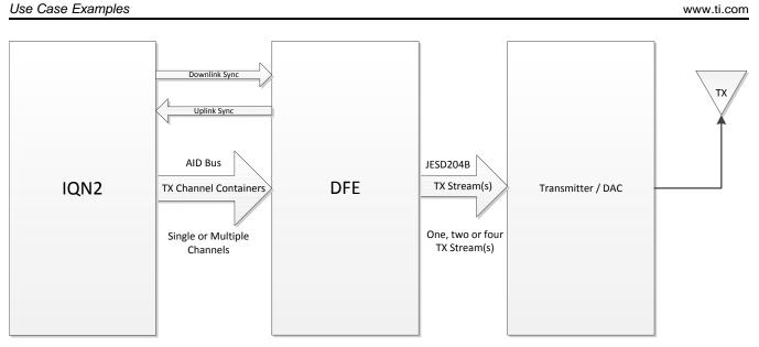
Figure 1-4. DFE TX Signal Processing
