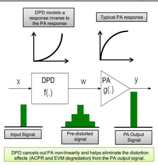
Figure 2-24. DPD Correction Showing TX Before Correction, Predistortion, and Post PA Response
