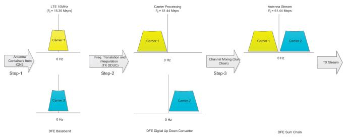
Figure 1-9. DFE TX Channel Processing
