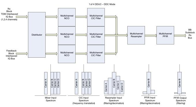
Figure 2-9. DDUC as a Digital Down Converter (Multicarrier Shown) Block Diagram
