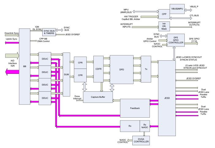
Figure 2-31. DFE Block Diagram for RX
