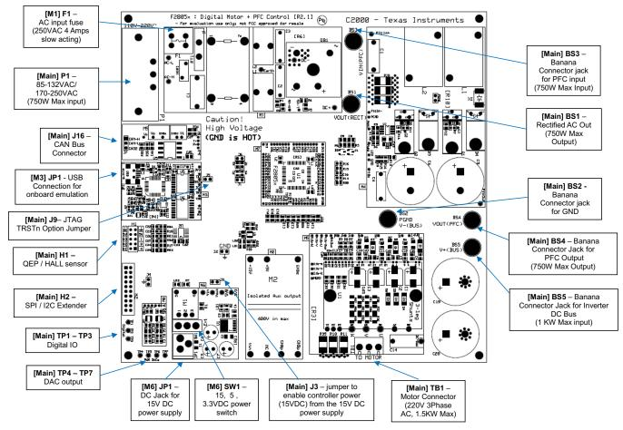
Figure 5. PCB Layout Diagram of the 1AXISMTR-PFC-5X Board
