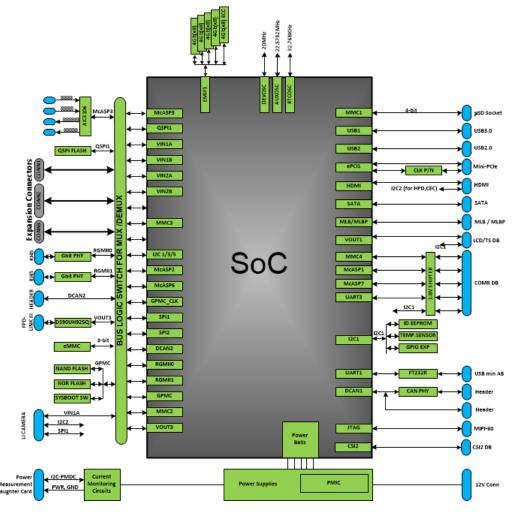
Figure 4. CPU Board Block Diagram
