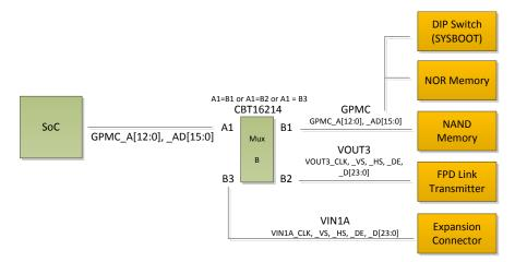
Figure 10. Mux Diagram for GPMC/VIN1/VOUT3
