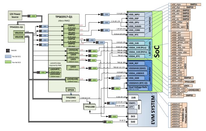
Figure 5. Power Distribution Block Diagram
