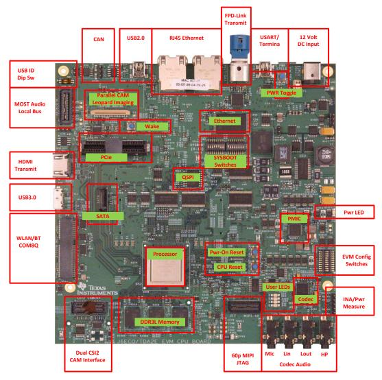
Figure 2. CPU Board – Front
