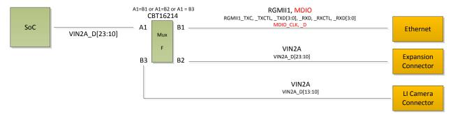
Figure 16. Mux Diagram for VIN2A and RGMII1
