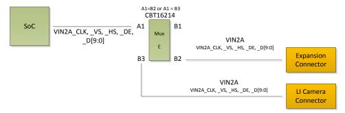
Figure 14. Mux Diagram for VIN2A and EMU
