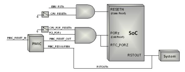
Figure 6. Reset Structure
