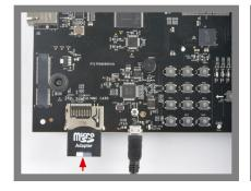
Prepare a Linux µSD card after downloading the software from www.ti.com/mysecuresoftware and following the instructions in the Processor SDK-EPOS Quick Start Guide. Insert the µSD card into the AM438x EVM as shown.
