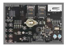
This EVM comes with a coin battery holder. A coin battery is not necessary for normal operation of the EVM. A coin battery (not included) can be inserted for testing ultra-low power (tamper-only) mode.
