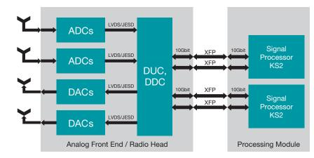
Figure 3: Proposed radar sytem with XFP interface
