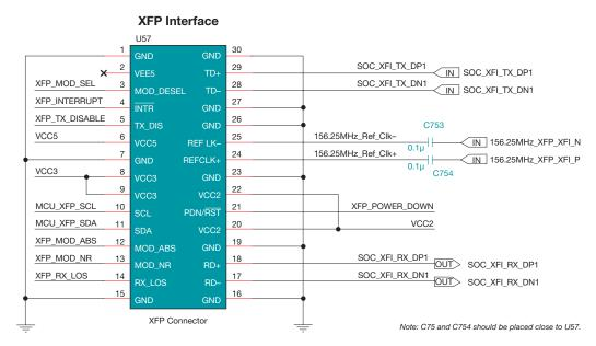
Figure 5: Typical electrical interface for XFI-to-XFP connector
