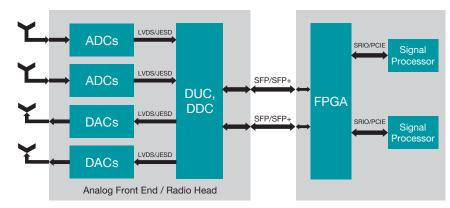
Figure 1: Conventional radar
