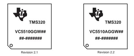
NOTE: Qualified devices are marked with the letters TMS at the beginning of the device name, while nonqualified devices are marked with the letters TMX at the beginning of the device name.
