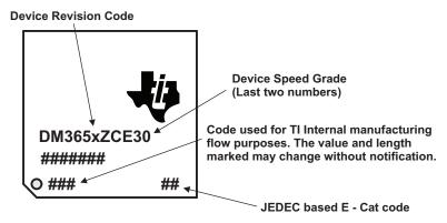
Figure 2. Example 2, Device Markings for TMS320DM365 (ZCE)
