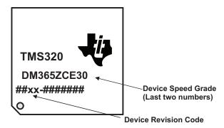
Figure 1. Example 1, Device Markings for TMS320DM365 (ZCE)
