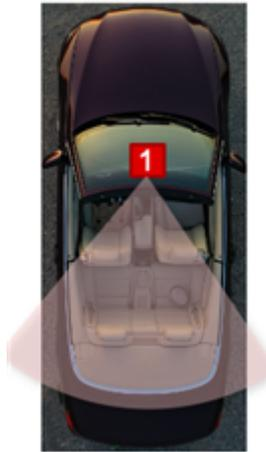
**Figure 2. Front Dash Placement Sensing**
