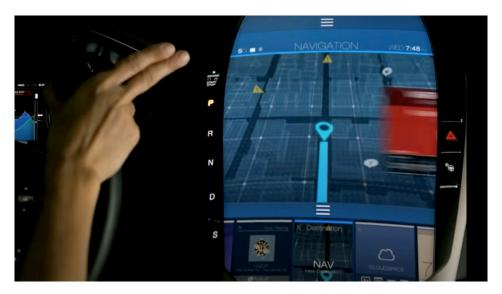
With a swipe of the hand, gesture detection gives drivers a new way to control in-cabin climates, lighting, windows, infotainment systems and more. There are currently several options for adjusting various comfort and convenience functions in the cabin. However, manipulating the buttons, knobs and especially touchscreens requires drivers to divert their eyes.
