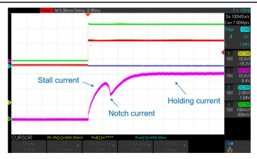
Figure 3. Output Current Profile of a Solenoid Actuator Captured by Current Sense of TPS274160
