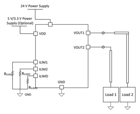
Figure 2. Dual-channel High-side Switch, TPS272C45
