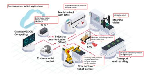
Figure 1. Illustration of Power Switches in Different Factory Automation Equipment
