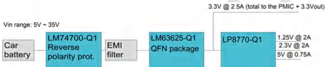
**Figure 2. Typical power block diagram of a radar system**
