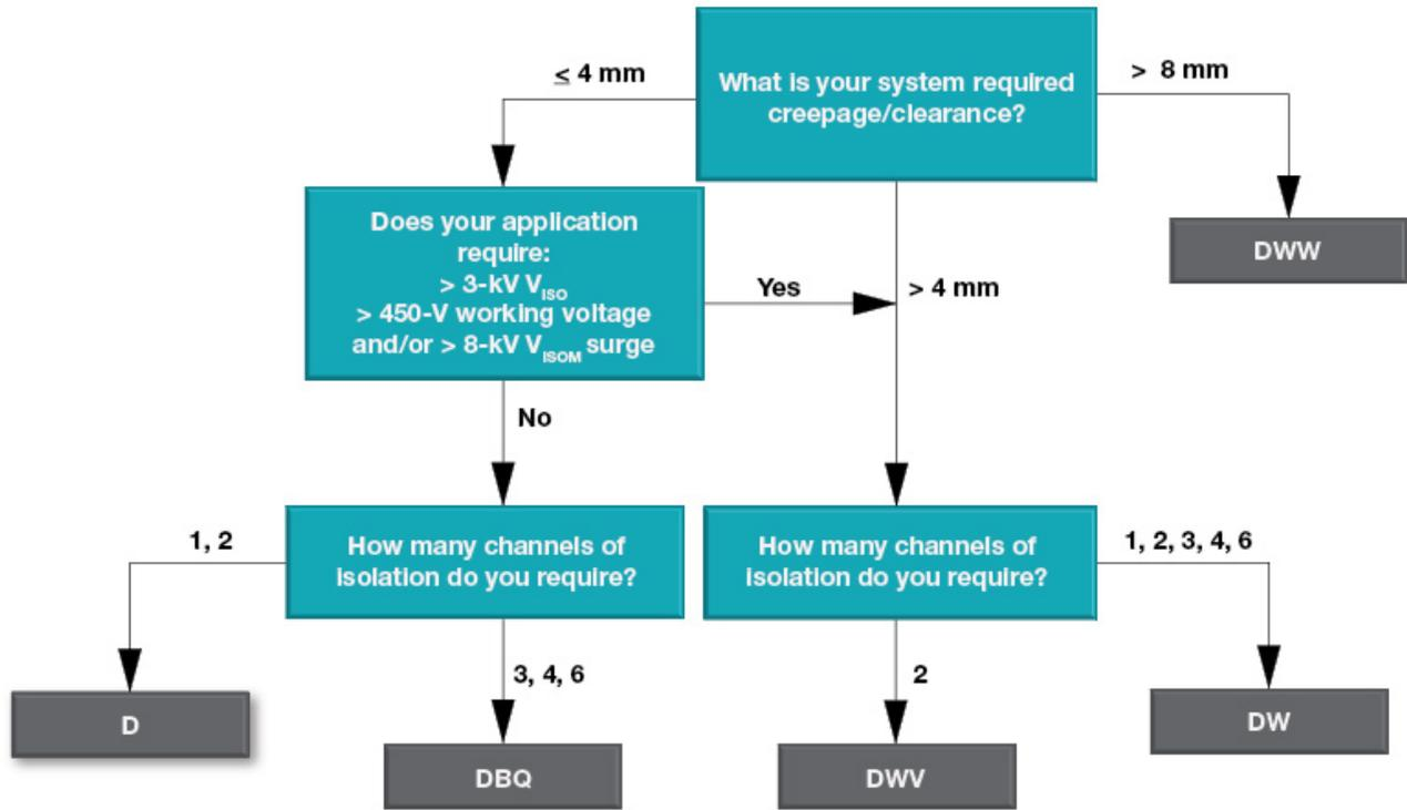
Figure 2. TI Digital Isolator Package Type Selection Flowchart
