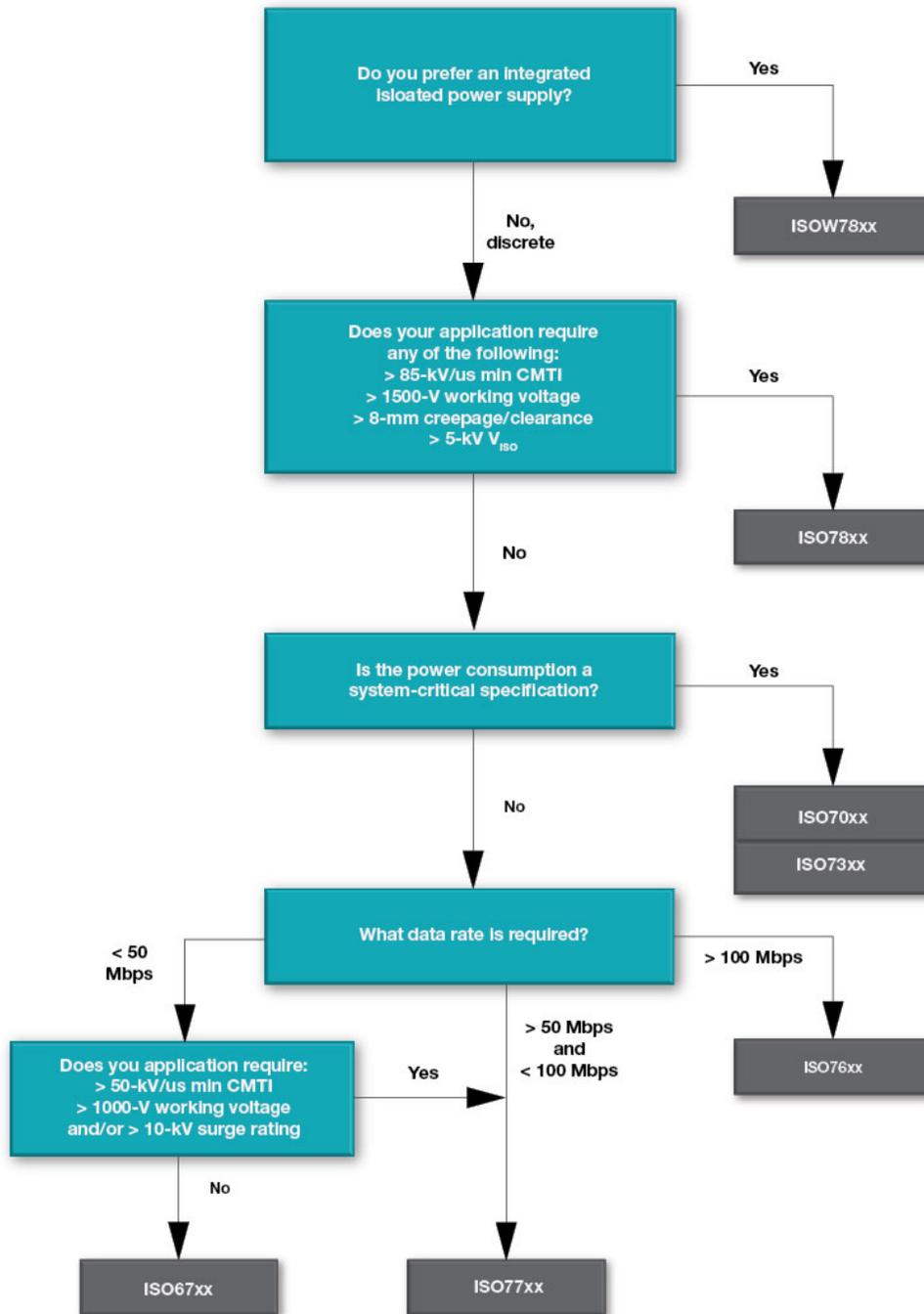
Figure 1. TI Digital Isolator Selection Flowchart
