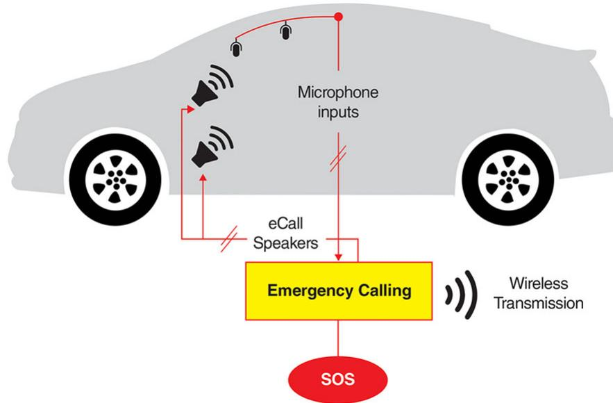
**Figure 3. How an eCall System Works**
