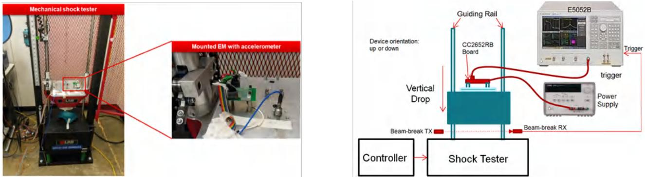
Figure 1. Mechanical shock test setup and test setup block diagram
