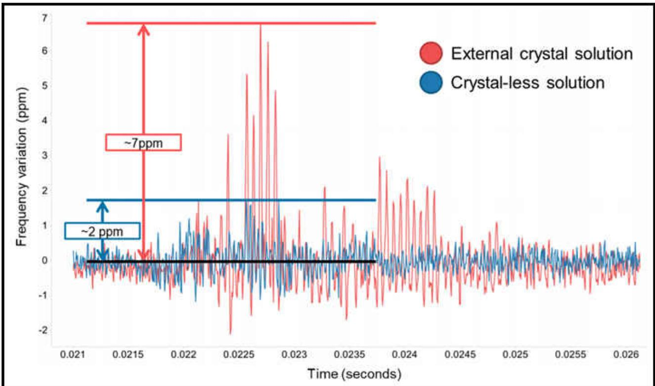
Figure 2. Comparing the maximum radio (2,440 GHz) frequency deviation (parts per million) induced by mechanical shock on both BAW and crystal devices
