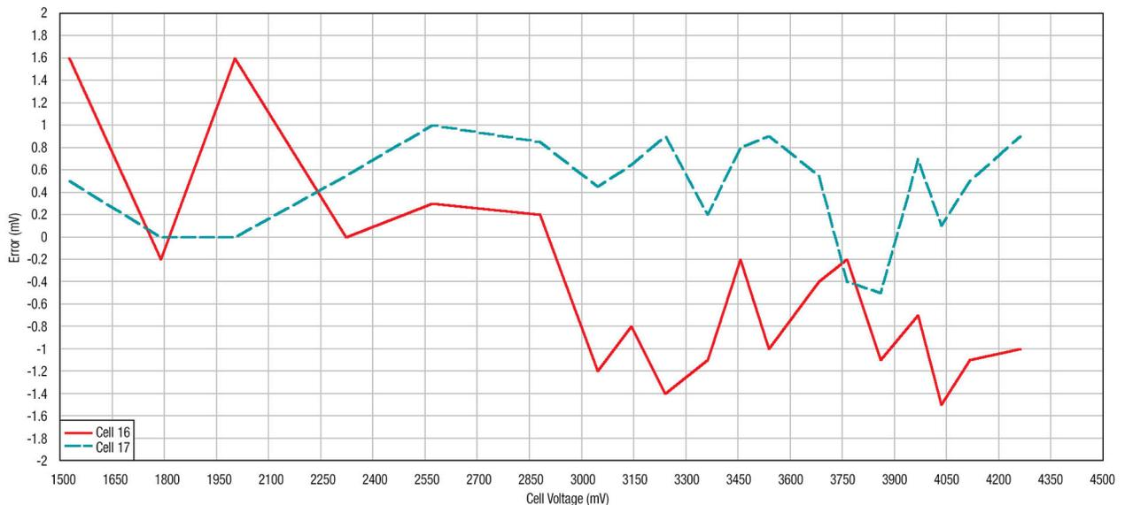
**Figure 4. 16th and 17th Cell Voltage Accuracy (at 25°C)**
