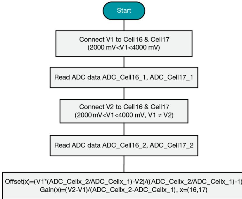
**Figure 3. Two-point Calibration Process**
