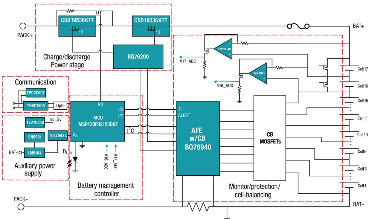
Figure 1. 16S-17S Battery Pack Block Diagram
