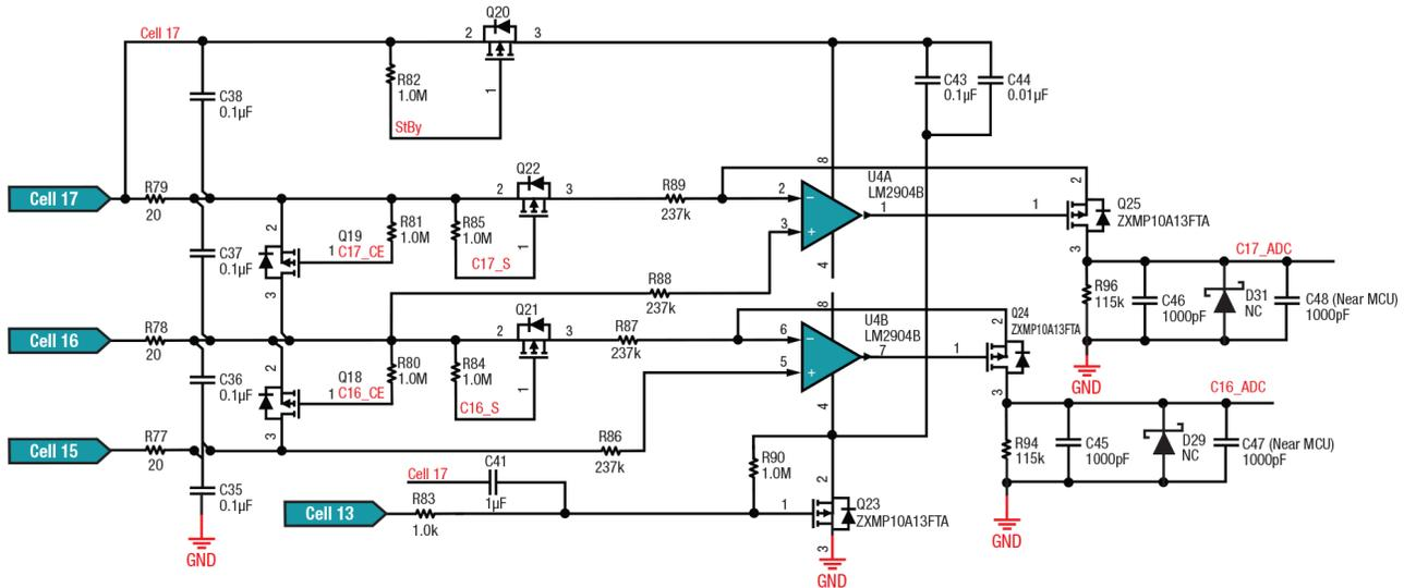
**Figure 2. Diagram of the Discrete Circuits for the Two Upper Cells**
