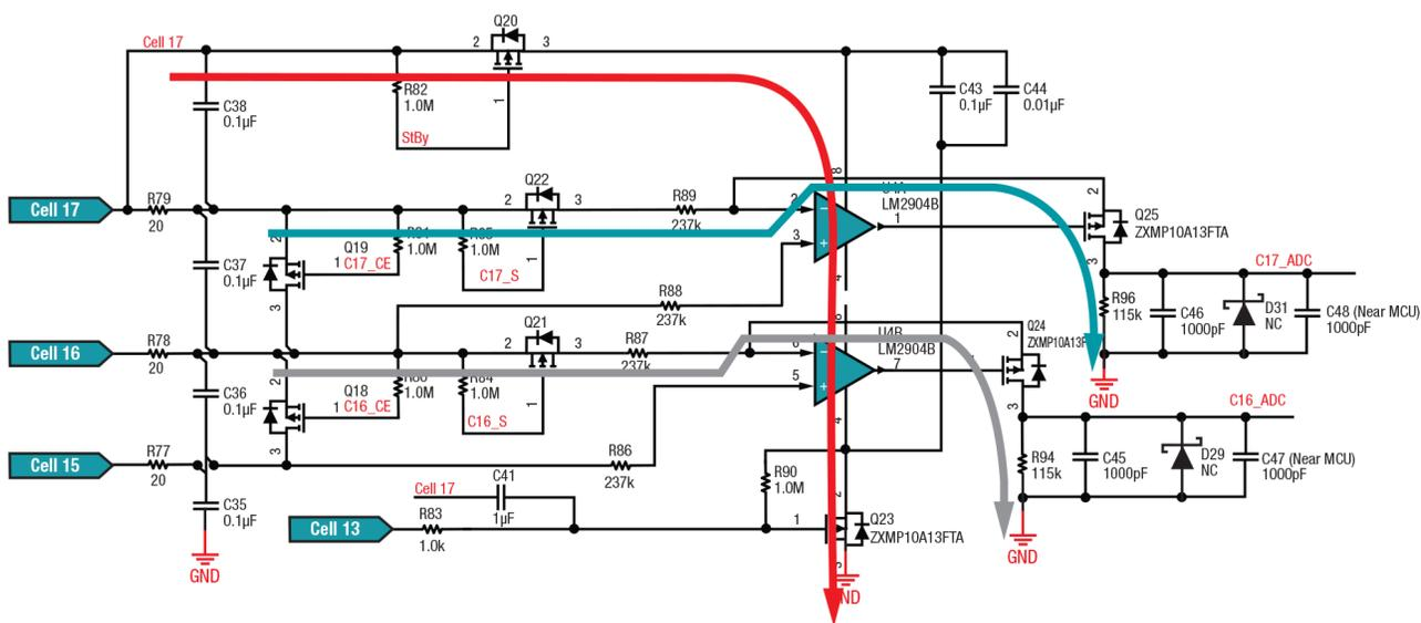
Figure 5. Diagram of the Current Paths of the Discrete Circuit
