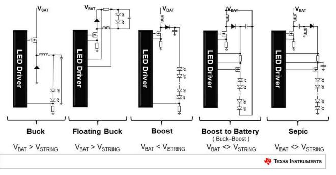
Figure 2. Basic schematics of common DC/DC LED driver topologies
