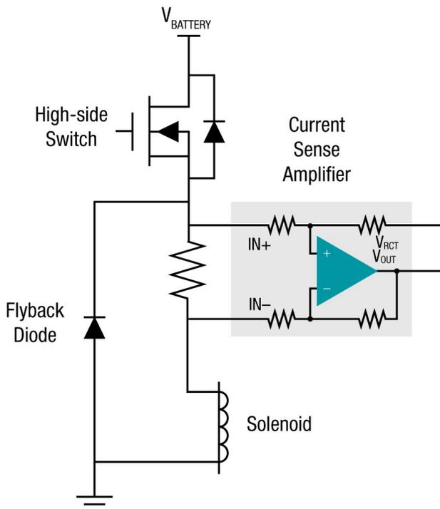
**Figure 1. Solenoid current measurement**
