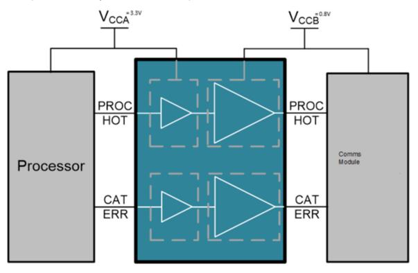
Figure 4. GPIO Level-translation Example Using the SN74AXC2T45
