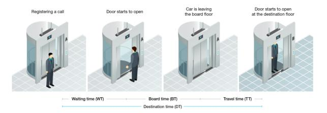
Figure 1. Time segments of elevator destination time
