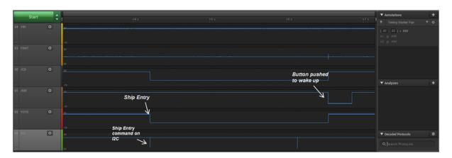
Figure 6. Ship Mode Entry through I2C Command
