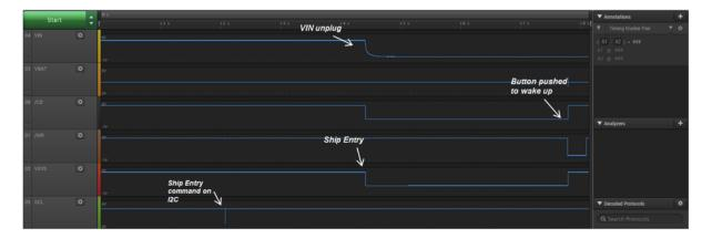
Figure 3. Illustration of Ship Mode at a Factory Production Line
