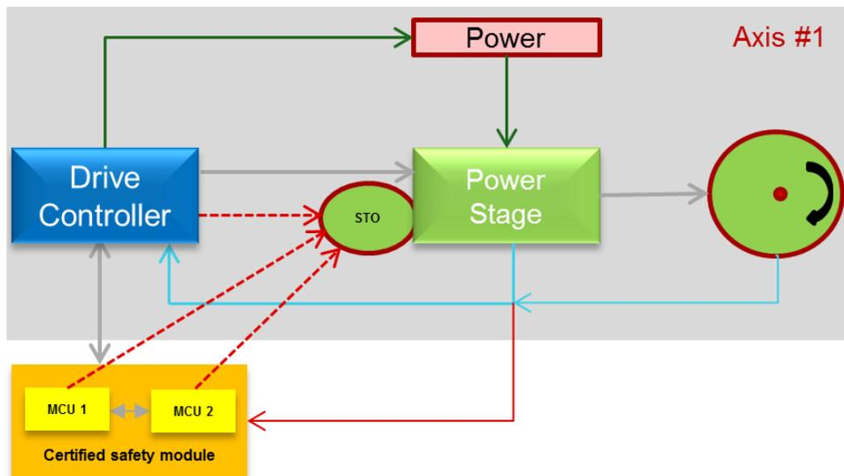
**Figure 1. Two-channel functional safety module example**
