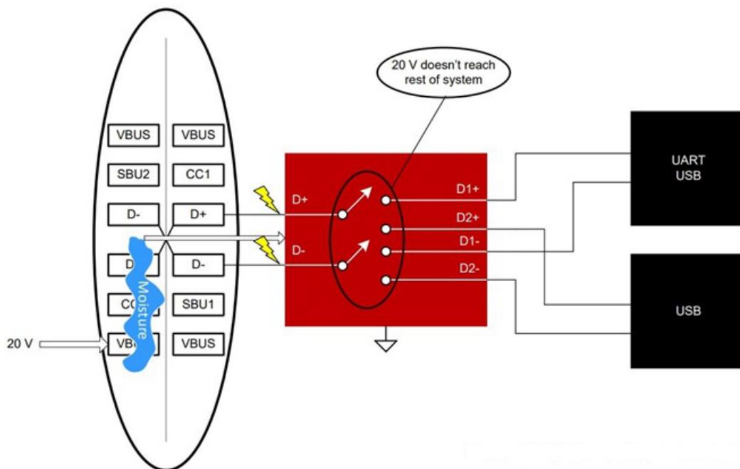
**Figure 2. The TS5USBC41 Protecting the System During an Overvoltage Event**
