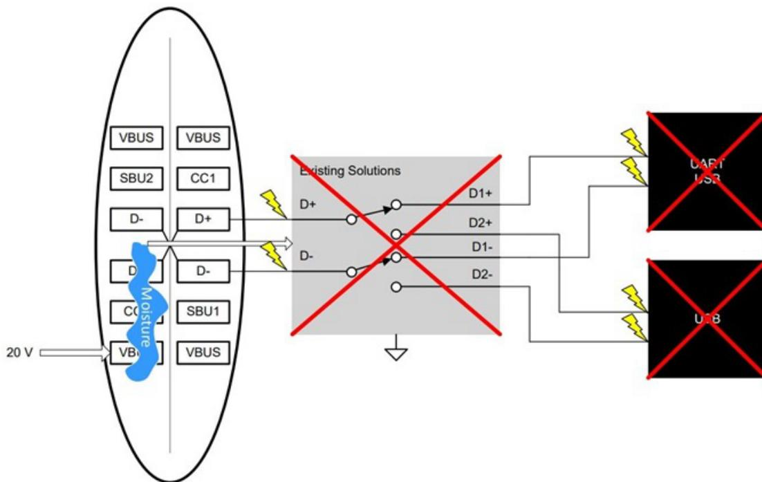
Figure 1. A Traditional USB Switch without OVP
